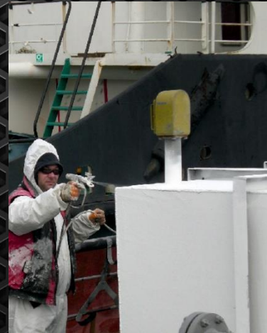
Isolation of the cab and technological storage tanks for petroleum products on a river barge
