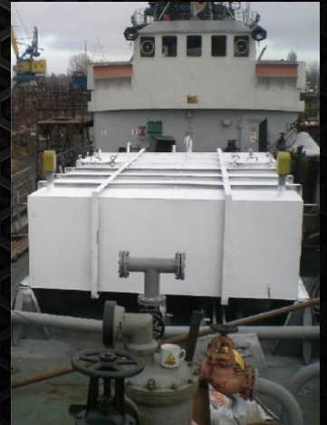
Isolation of the cab and technological storage tanks for petroleum products on a river barge
