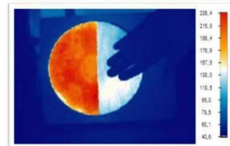
Photo of the electric heater made by thermal camera, one half of the heater is coated with Bronya heat insulation
