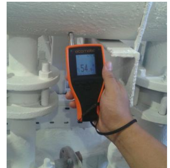
Accurate measurements of the Bronya can be made Elcometer® 319 or tactile test
