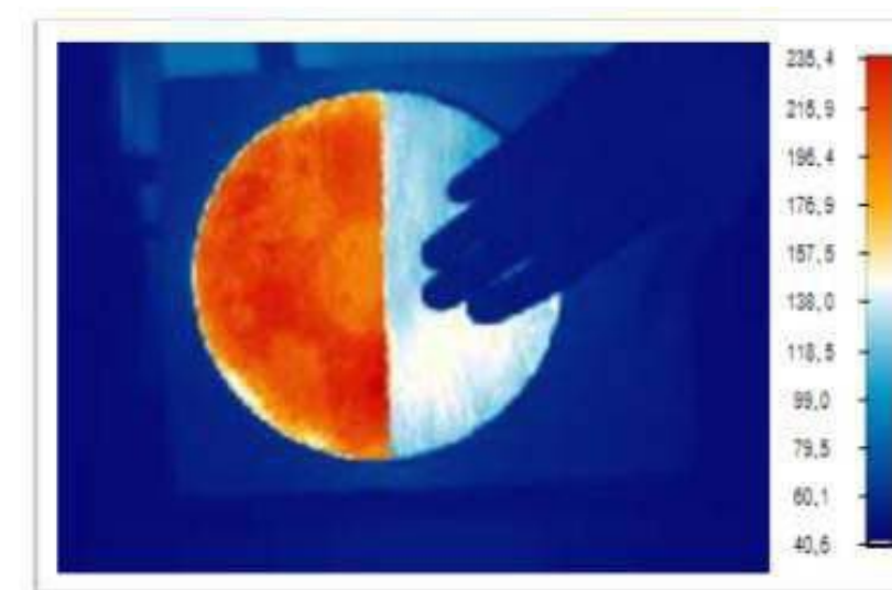
Photo of the electric heater made by thermal camera, one half of the heater is coated with Bronya heat insulation
