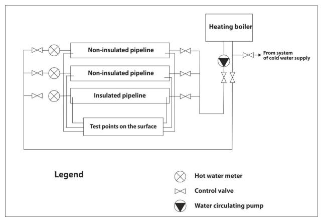
Fig. 1 – Basic scheme of the test facility
