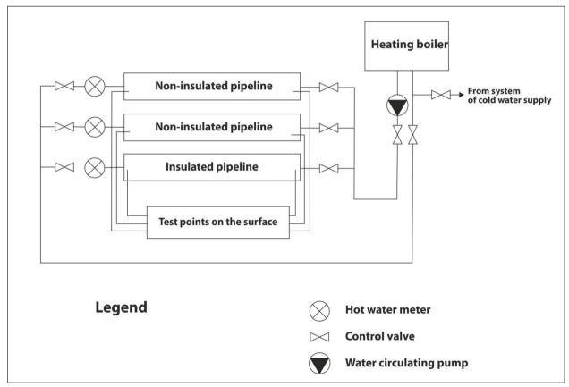
Fig. 1 – Basic scheme of the test facility
